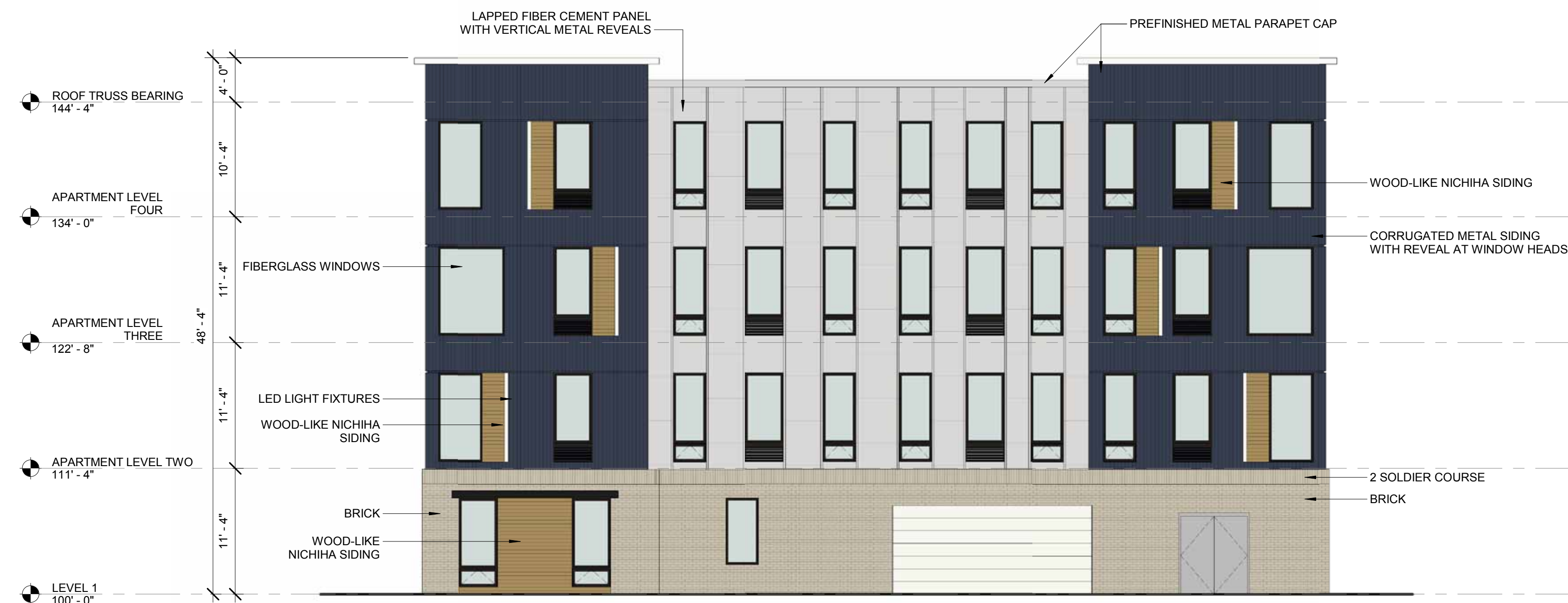
4 NORTH EXTERIOR ELEVATION 1/8" = 1'-0"
