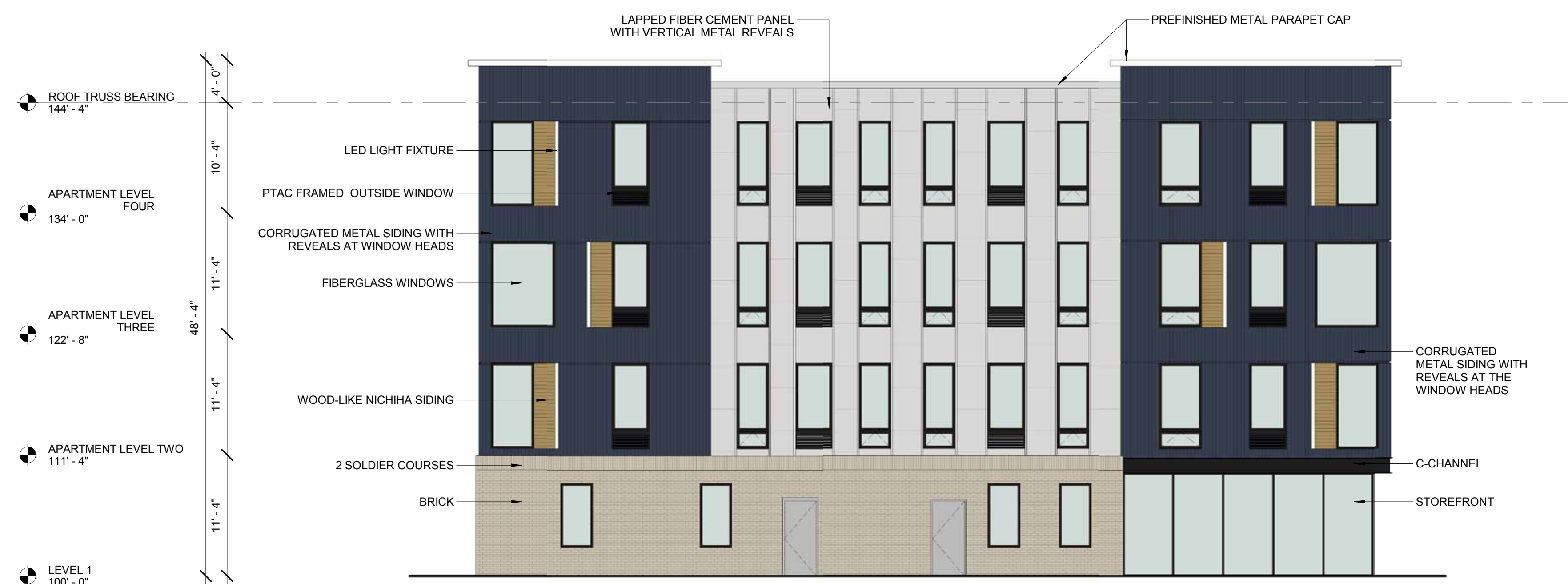
3 SOUTH EXTERIOR ELEVATION 1/8" = 1'-0"
