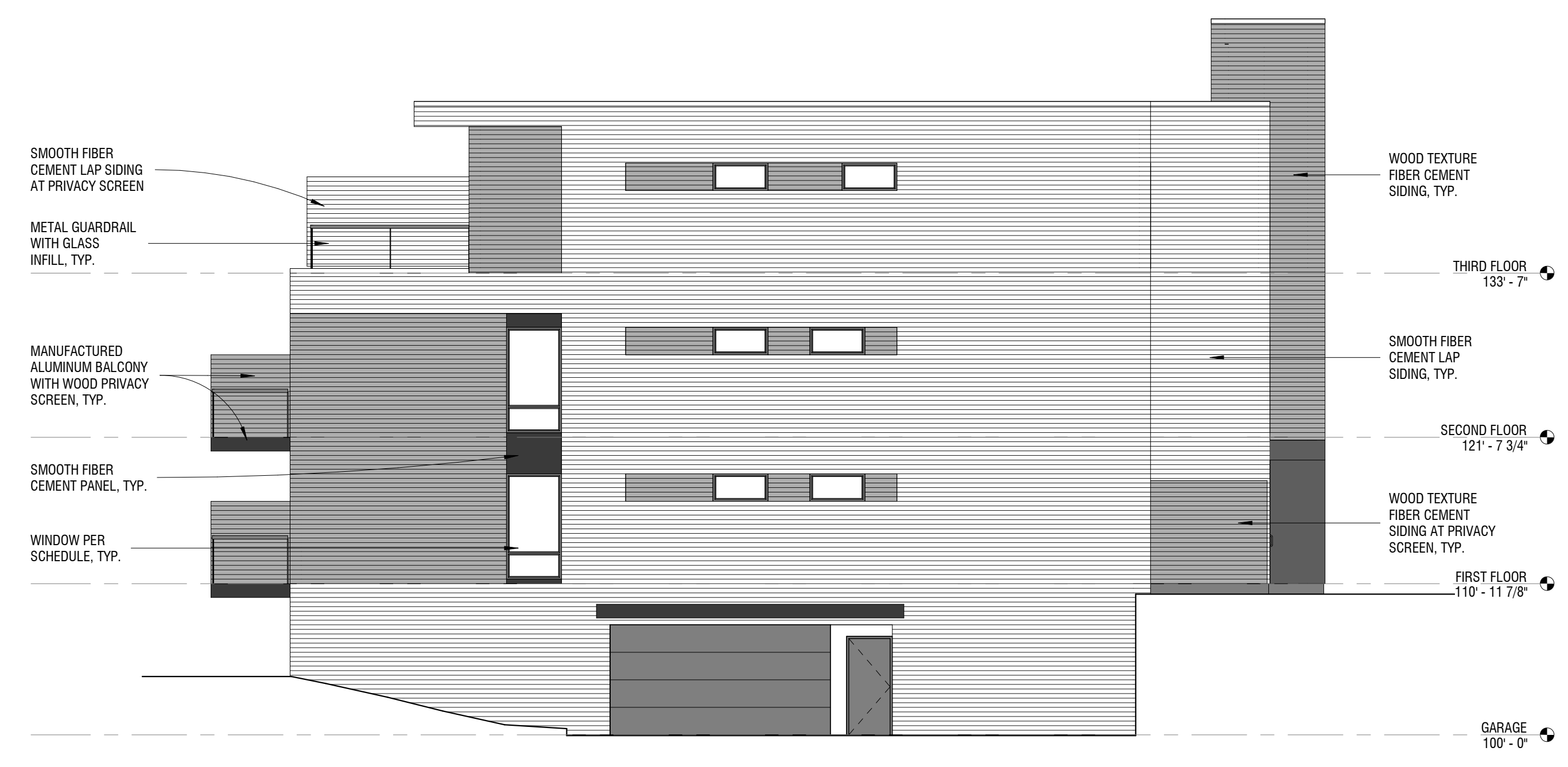
2 EAST ELEVATION - BUILDING B 1/8" = 1'-0"
