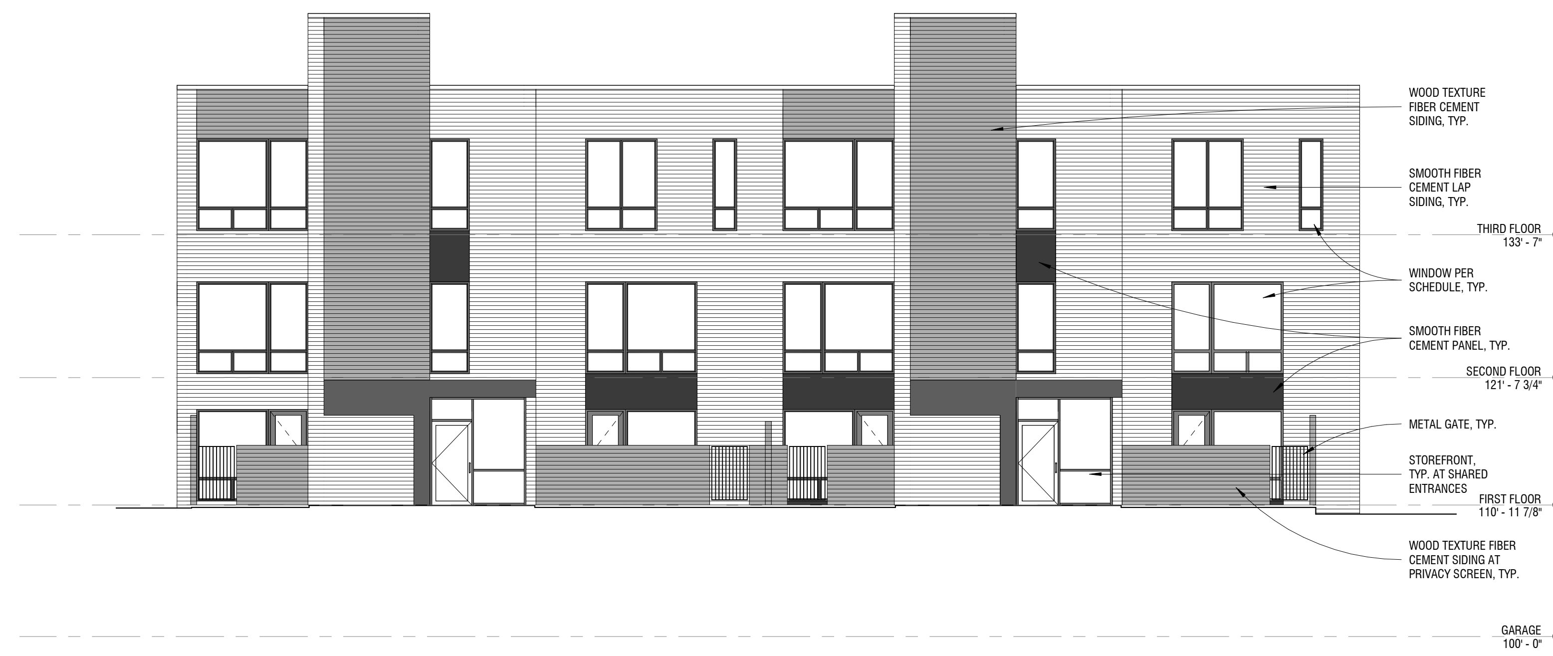
1 NORTH ELEVATION - BUILDING A 1/8" = 1'-0"
